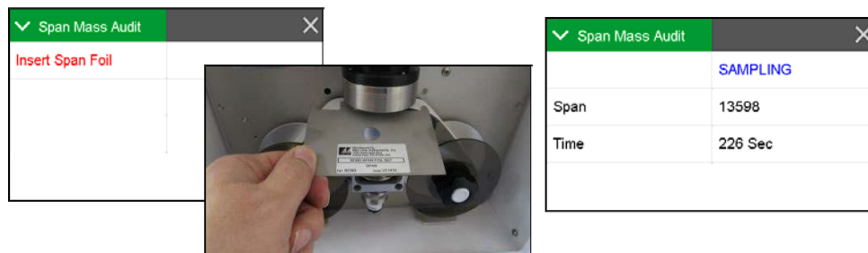
Figure 10-9. Starting the Span Test
