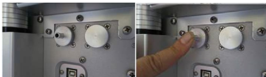
Figure 10-3. Sheath Air Inlet Location and Covered
