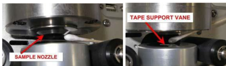
Figure10-7. Cleaning the E-BAM PLUS Nozzle and Vane with a Cotton-Tipped Applicator
