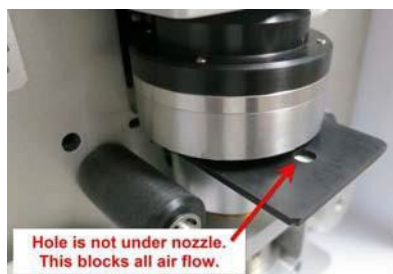
Figure 12-1. Nozzle Sealing Tool Lower System Test
