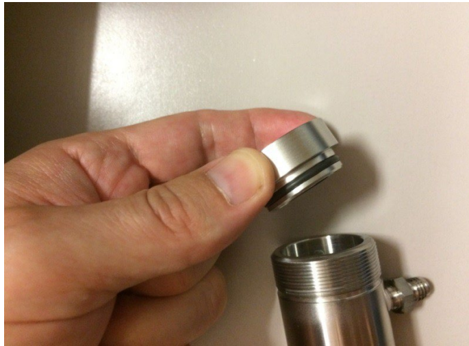
Figure 11-17. Mirror is housed in a protective holder.
