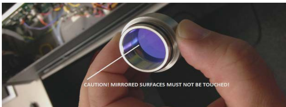
Figure 11-18. Mirror with Reflective Surface side showing.
