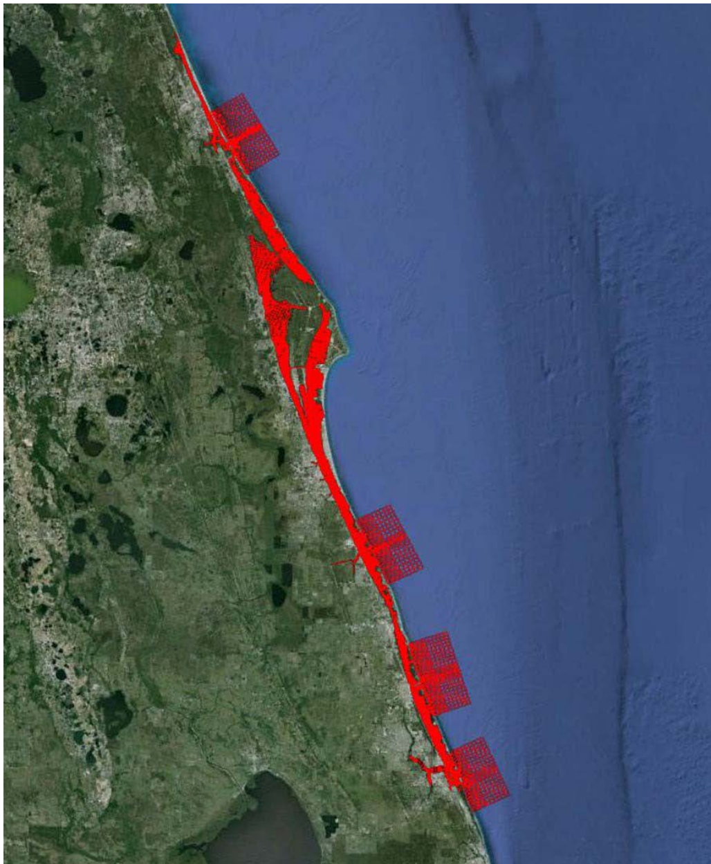
Figure 3-8. Extent of the SJRWMD's EFDC model grid of the IRL. .
