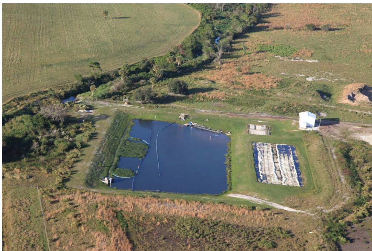
Figure 1. The Nubbin Slough HWT system looking toward the north. The mixing chamber and inflow manifold are at the northeast corner of the pond, and the outflow riser is at the southwest corner (left foreground). The inflow region limerock bed is situated to the right of the pond. Early in 2015, an additional limerock bed (not shown in this photo) was installed at the system outflow, adjacent to the outflow riser.
