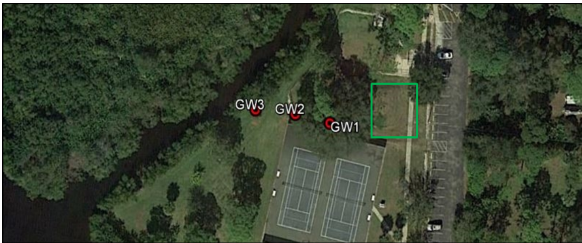
Figure 5. Groundwater monitoring wells (GW1-GW3) in Judd Community Park located within the Hancock Creek watershed on the western side of North Fort Myers, FL; the approximate location of the septic tank drainfield is indicated by the green square.
