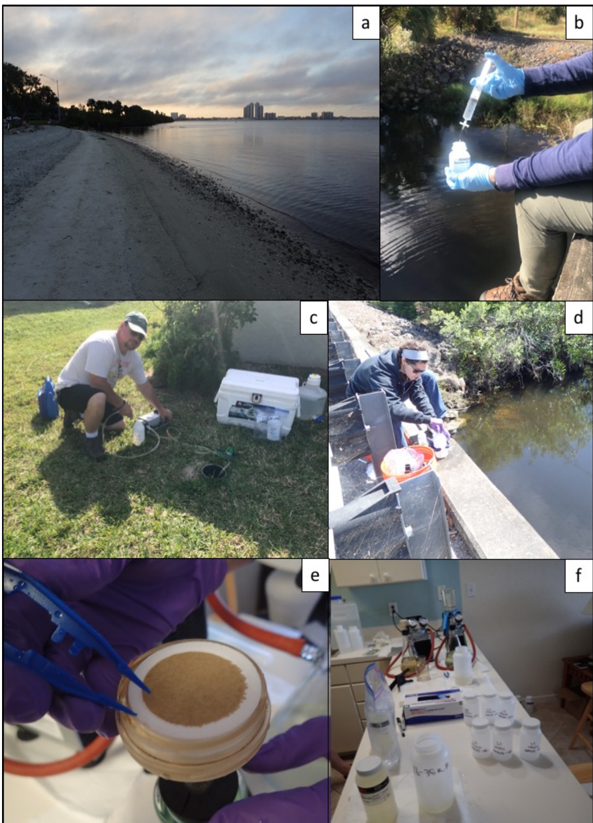
Figure 12. Images from the study including, a) North Shore Park at sunrise, b) hand-filtering a surface water sample, c) pumping groundwater from a monitoring well, d) collecting water samples, e) removing a groundwater filter from a vacuum pump, and f) the temporary laboratory set up for HBOI sample processing.
