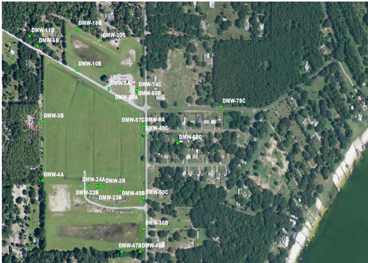
Figure 5-12. Locations of observation wells of hydraulic head in surficial aquifer.
