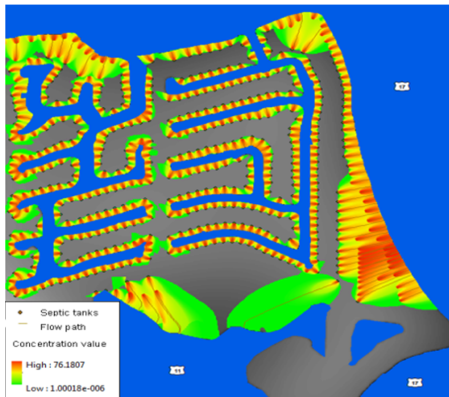
Figure ES-3. Simulated flow paths and nitrogen plumes from the removed septic systems in Seagate Harbor. The flow paths are the shortest among the seven modeling sites.
