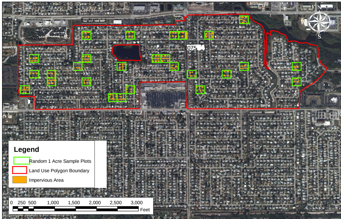
Figure 1. Example of Sampled Impervious Area Delineation for Medium Density Residential Polygon.
