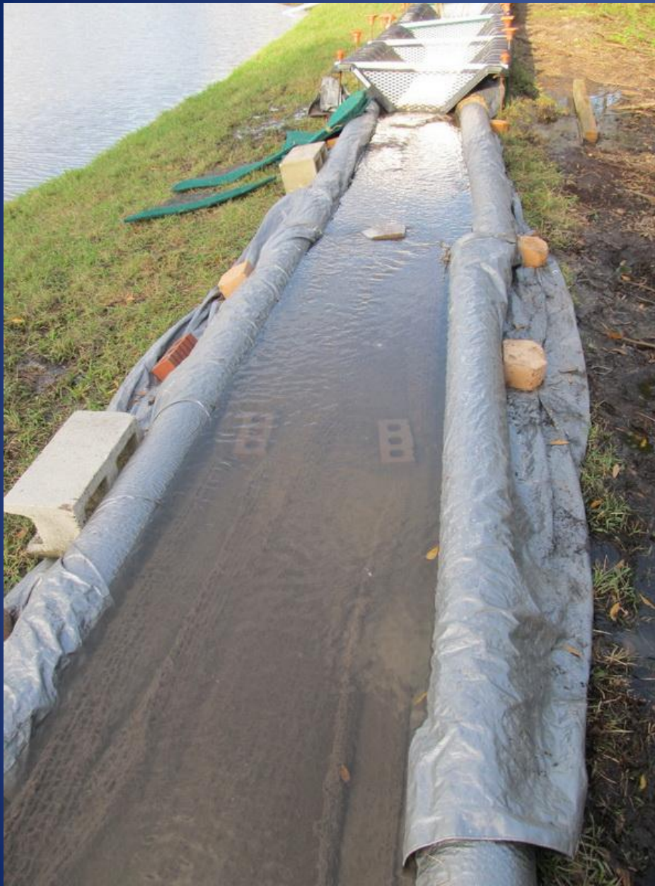
Accelerated Capture Of Medium/Small Floc Particles On Jute Fabric
