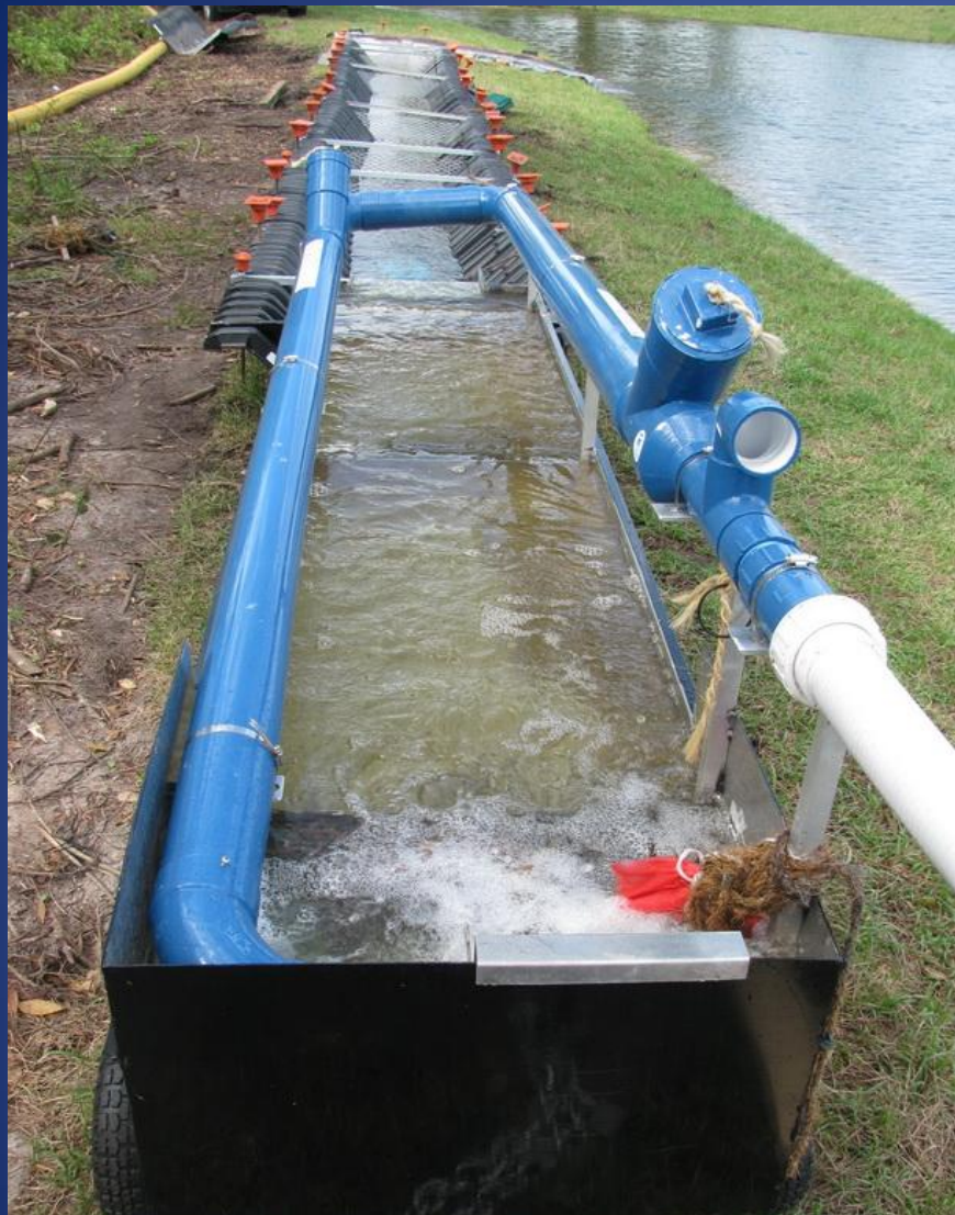
Double Mixing Chambers Using Air Injection Technology *Extremely Efficient PAM Mixing System
