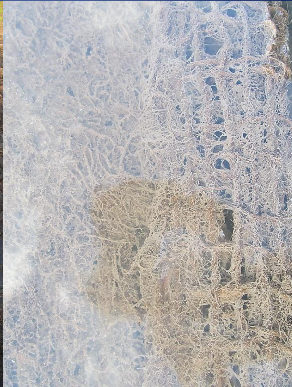
Accelerated Capture Of Medium/Small Floc Particles On Jute Fabric
