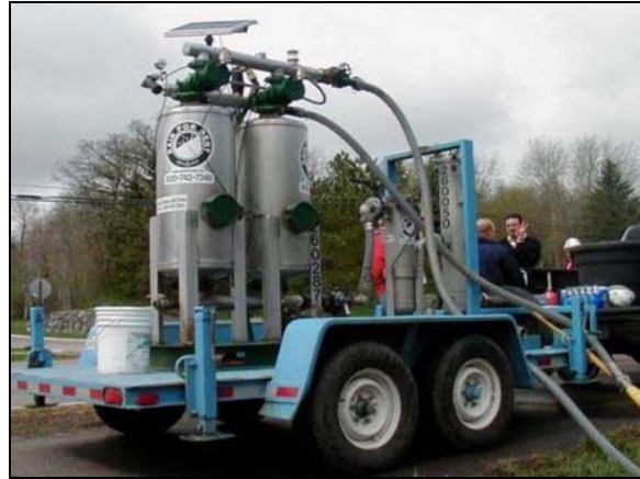
Sand Media Particulate Filter
