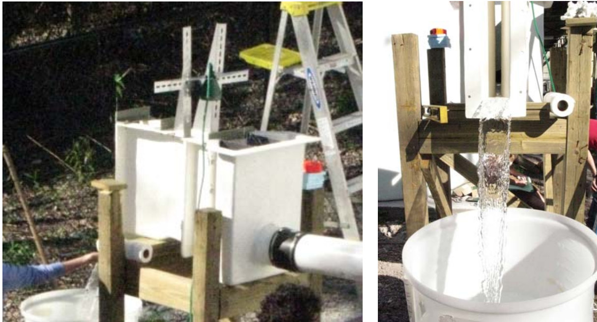
Figure 9 Parshall Flume calibration set-up
