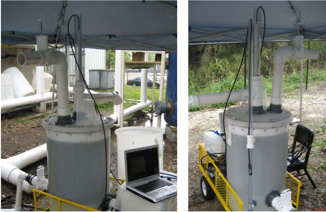
Figure 11 Hydraulic conductivity set-up and testing for engineered soil media
