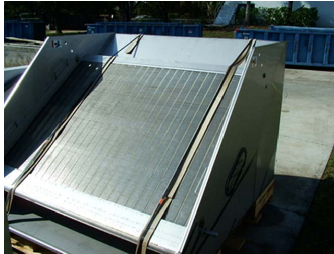
ADDITIONAL STATIC SCREENS INSTALLED AT HEADWORKS
