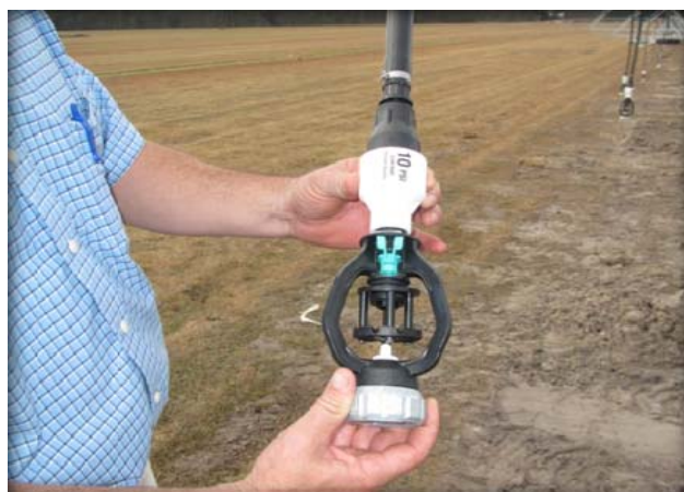
DROP NOZZLE TO MINIMIZE WIND DRIFT AND EVAPORATIVE LOSS
