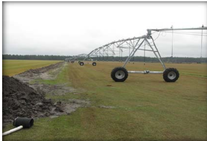
FIGURE 28: AGRICULTURE OVERHEAD PIVOT IRRIGATION ON SOD WITH FERTIGATION
