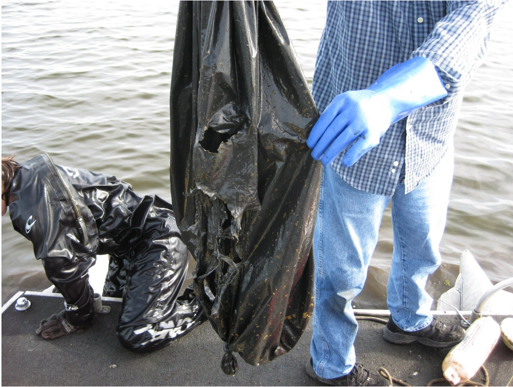
Figure 3-2. Example of Damaged Seepage Collection Bag.
