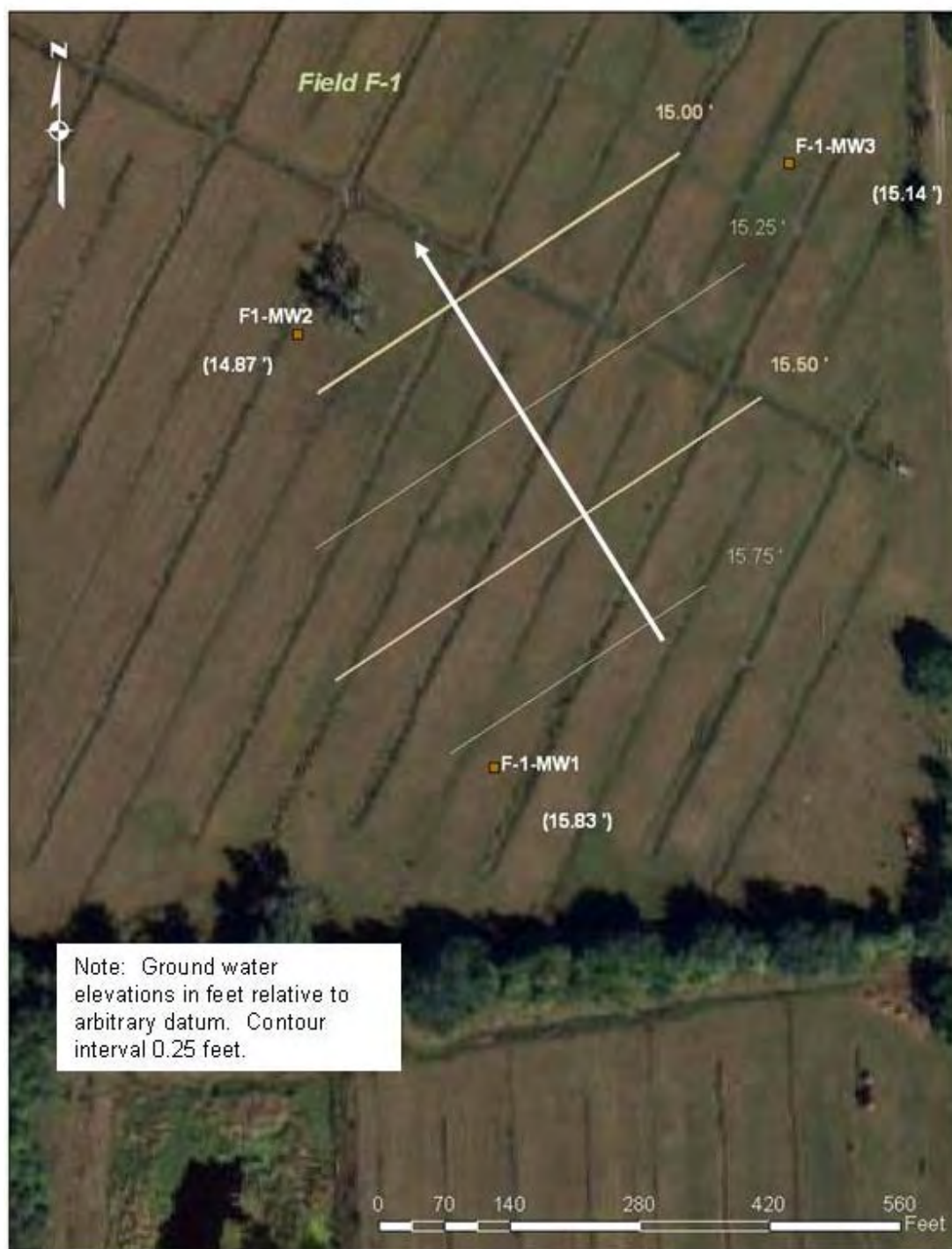
Figure 3 – Ground water contour map for Field 1, December 13, 2007.
