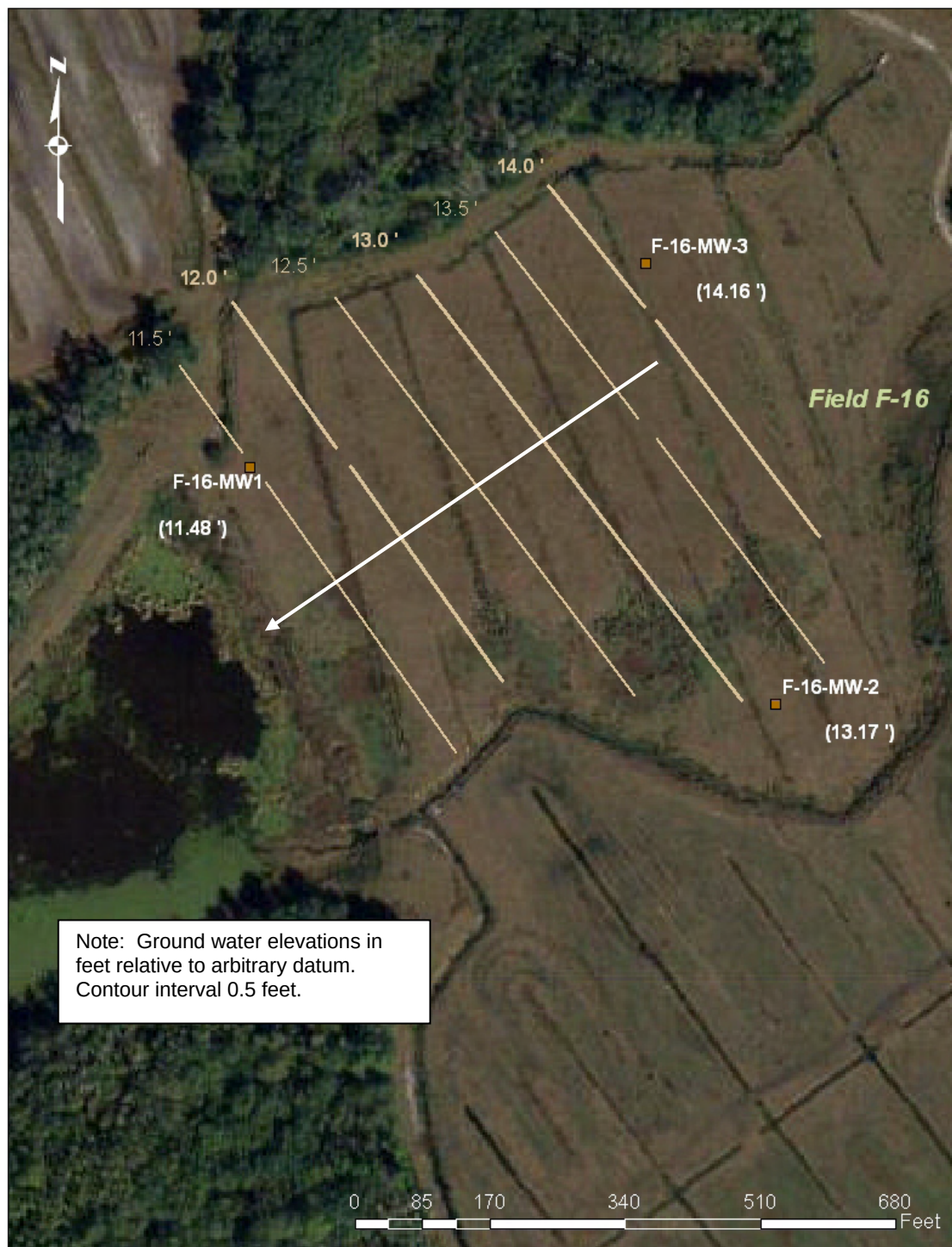
Figure 6 – Ground water contour map for Field 16, December 13, 2007.
