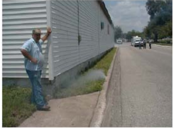
Illegal Connections to GRU Wastewater Collection System: Apartment Rain Gutter
