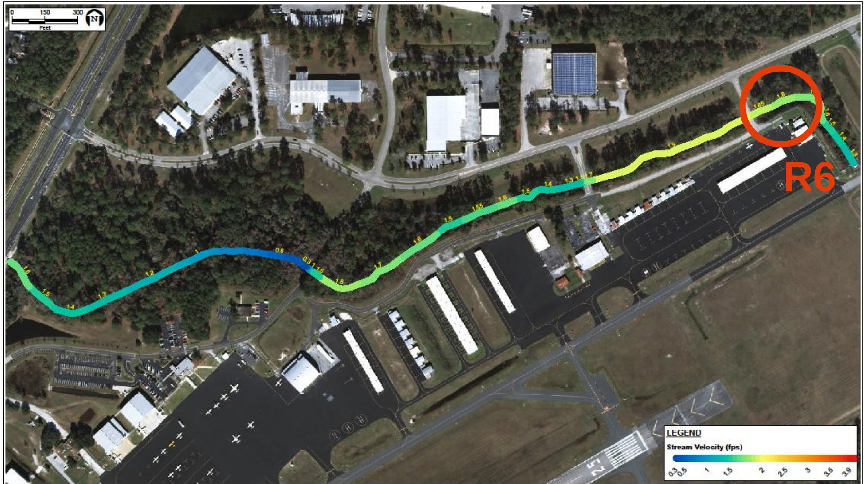
FIGURE 2. PROPOSED STREAM PROFILE MAXIMUM VELOCITIES WITH WEIRS LITTLE HATCHET CREEK
