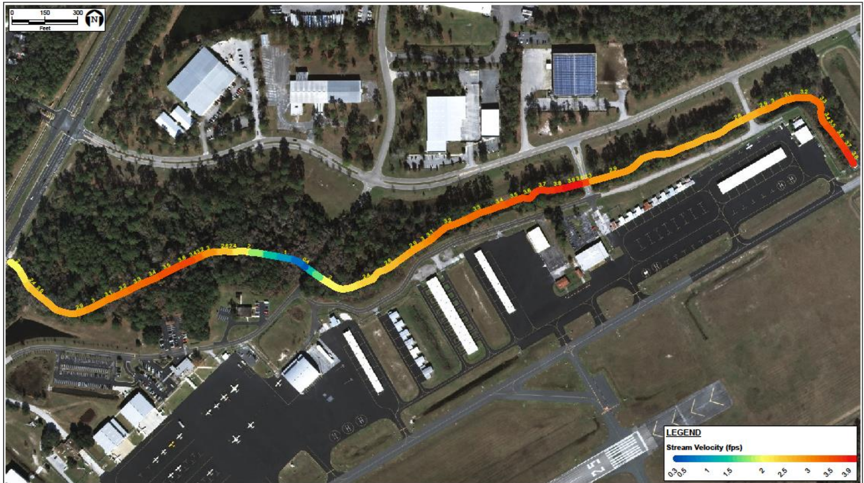
FIGURE 1. EXISTING STREAM PROFILE MAXIMUM VELOCITIES LITTLE HATCHET CREEK
