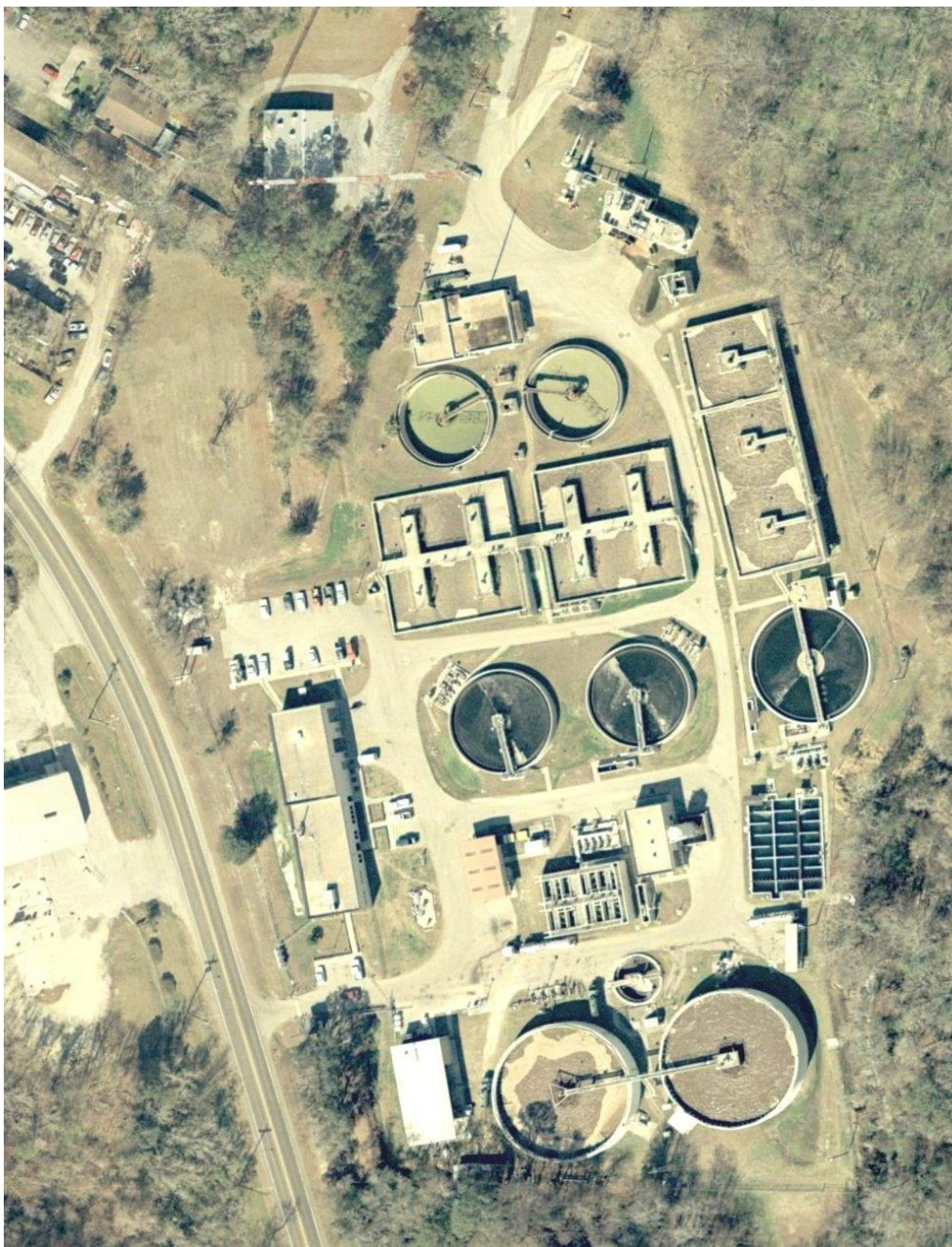
Figure M-6. Main Street Water Reclamation Facility aerial photograph illustrating two parallel advanced secondary treatment trains. Final chlorine contact chamber for disinfection is on the lower right of the photo and is the last point in the process before discharge to Sweetwater Branch.
