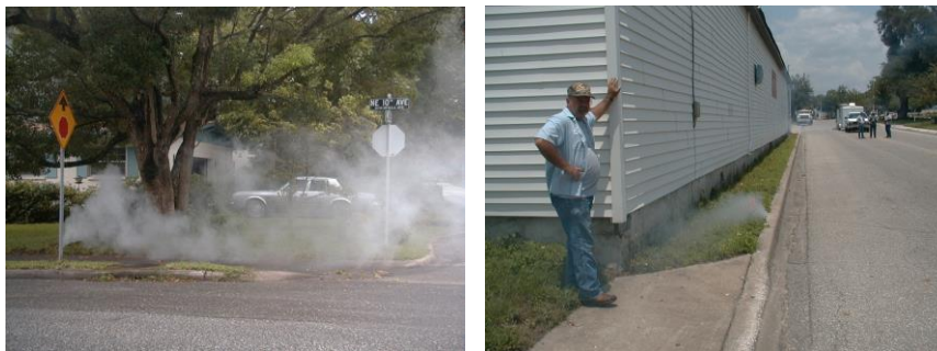
Figure 3.7. Smoke testing used to find I&I
