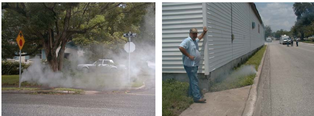
Figure 32 . Pictures of Smoke Testing Used to Find I&I
