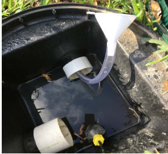
Figure 8 Sample Port #1 – Dye Injection via Funnel and Tubing
