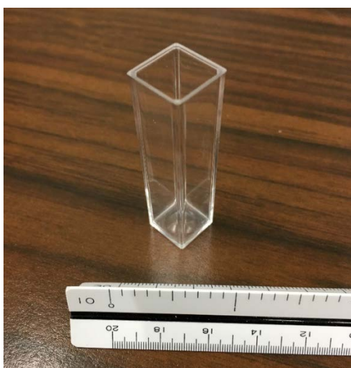
Figure 10 A 10 x 10 mm x 45 mm methacrylate sample cuvette (measure shown for scale).
