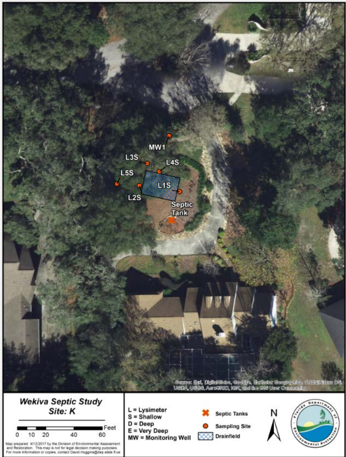
Figure 32. Septic system and monitoring devices at Site K
