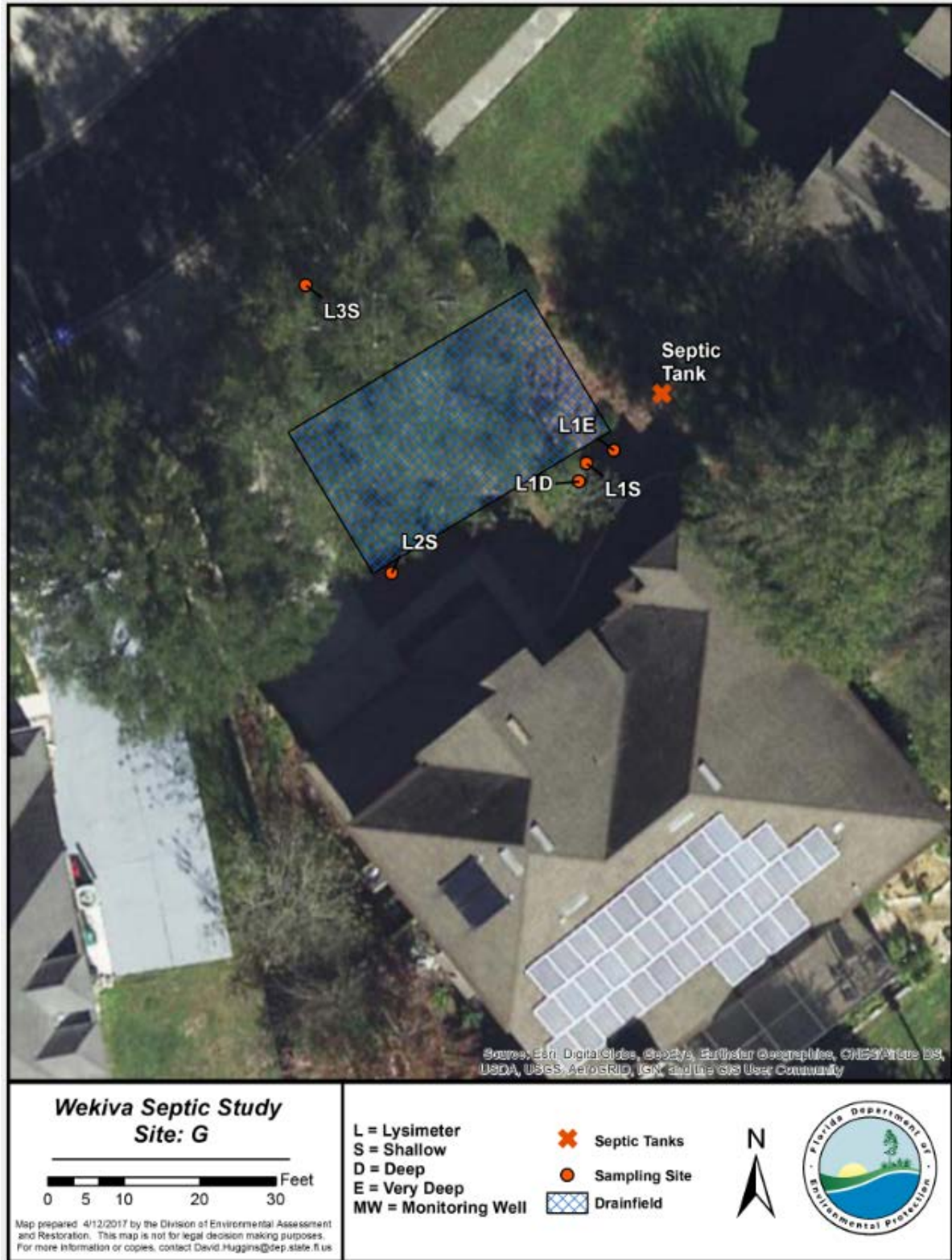
Figure 25. Septic system and monitoring devices at Site G
