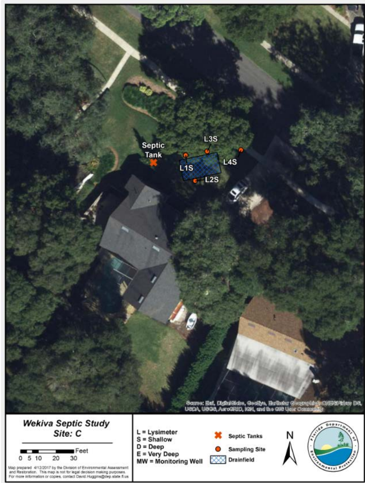
Figure 15. Septic system and monitoring devices at Site C
