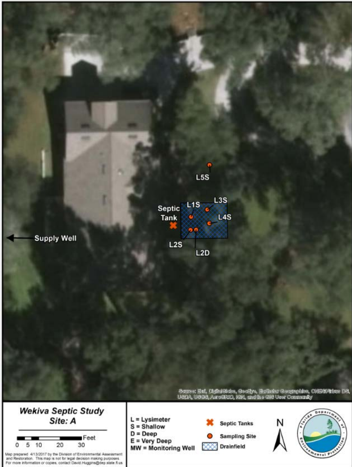
Figure 9. Septic system and monitoring devices at Site A
