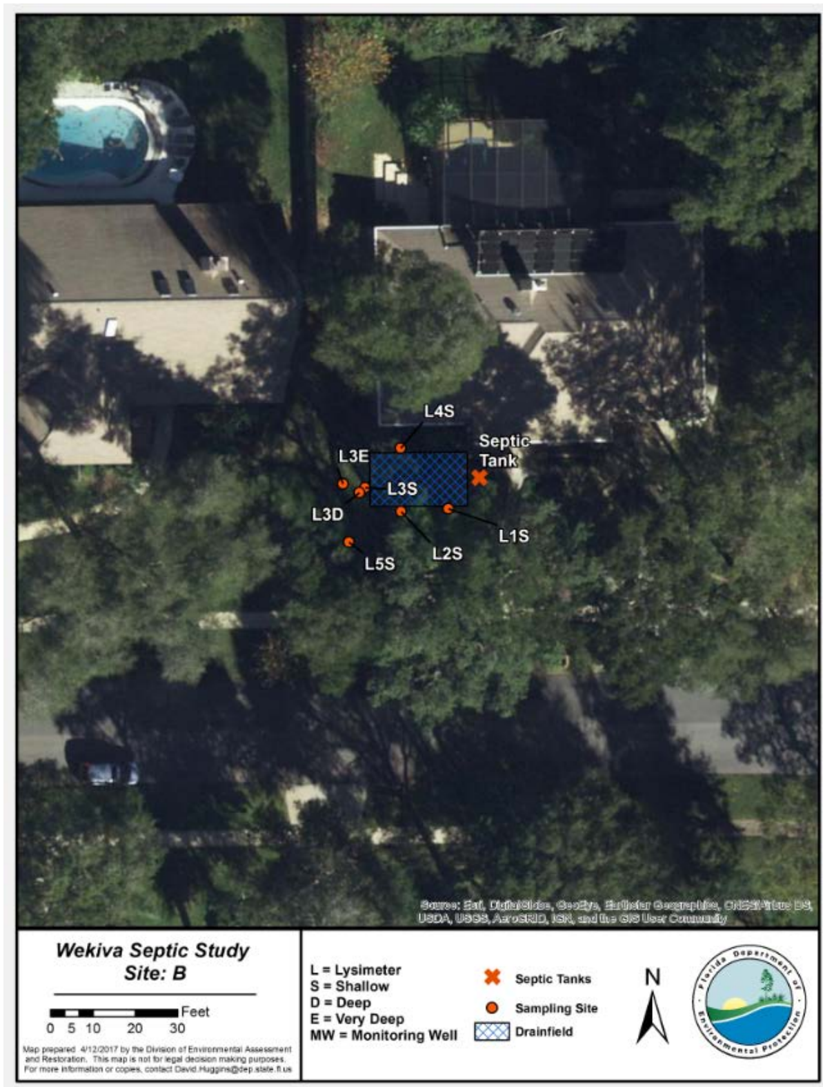
Figure 12. Septic system and monitoring devices at Site B
