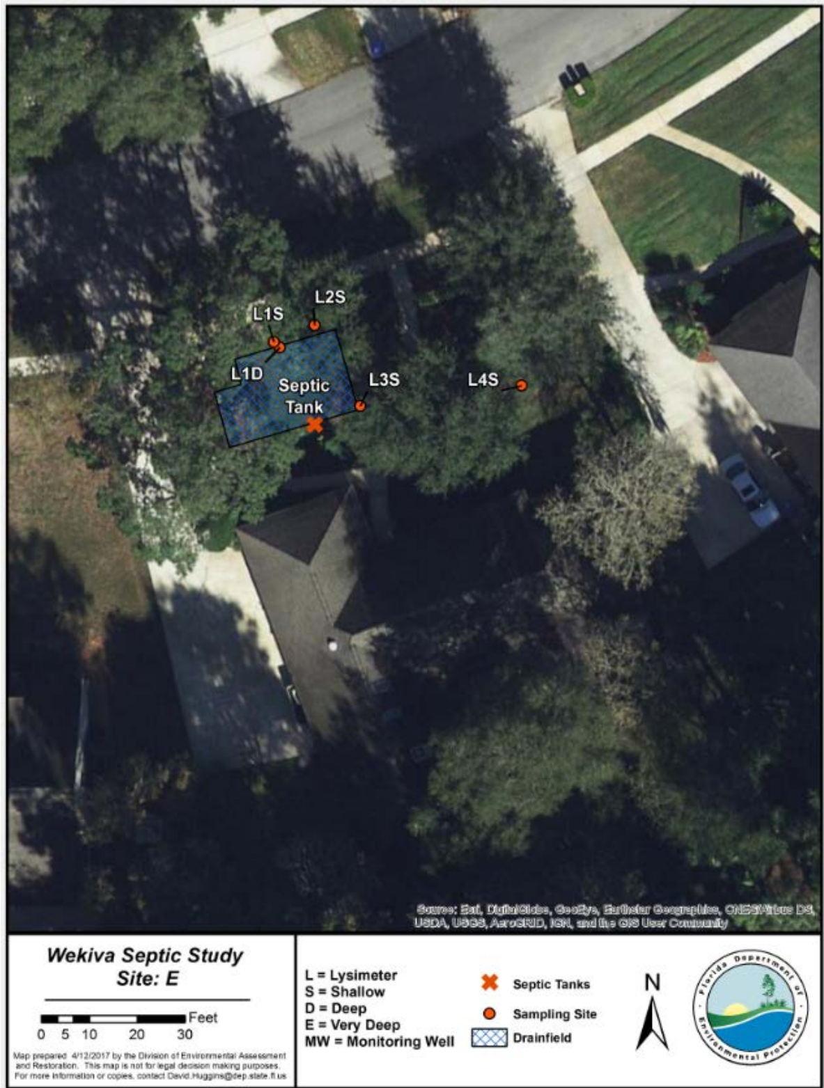
Figure 19. Septic system and monitoring devices at Site E
