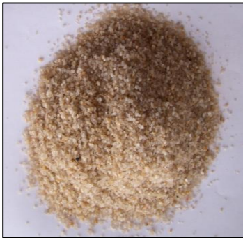
nitrification media: sand & expanded clay
