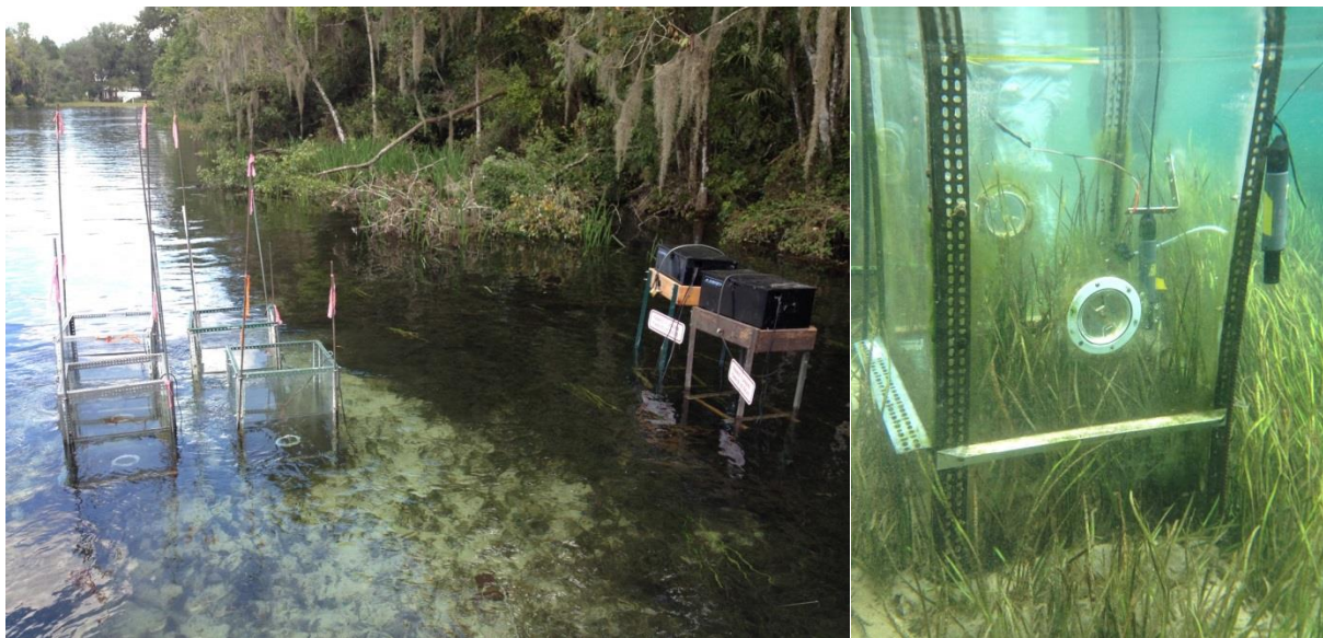
Figure 4-1. Set of four benthic chambers deployed in Rainbow River (left). Boxes in right of figure house batteries for pumps and sensors. Underwater view (right) showing HOBO sensors deployed inside and outside of chamber.
