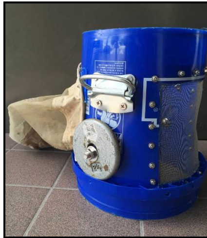
Figure 5 Photo of Custom-Made Modified Hess Sampler Used to Collect SAV and Benthic Macroalgal Samples
