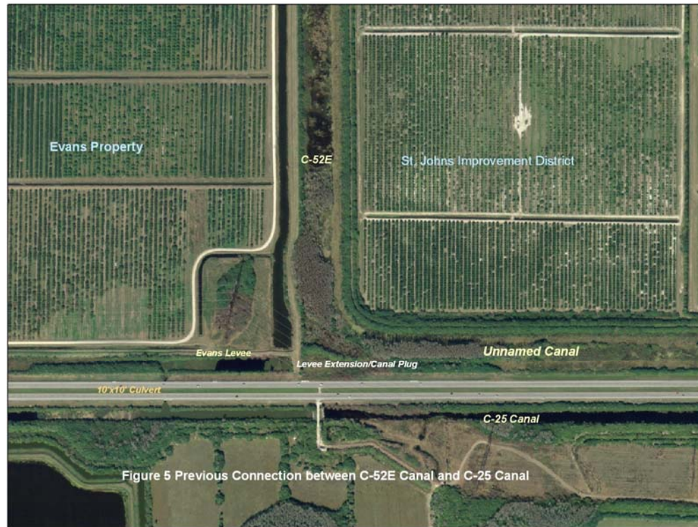
Figure 18. Historic (pre-1980) connection of the C-25 Extension Basin (via C-52 East) and C-25 (Figure 5 from Tai, 2009b).
