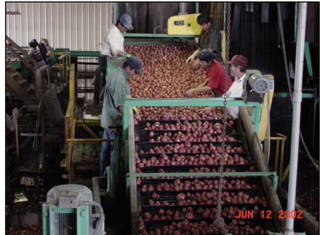
Figure 23 Potatoes in the processing line being presorted before entering the hydra cooler.
