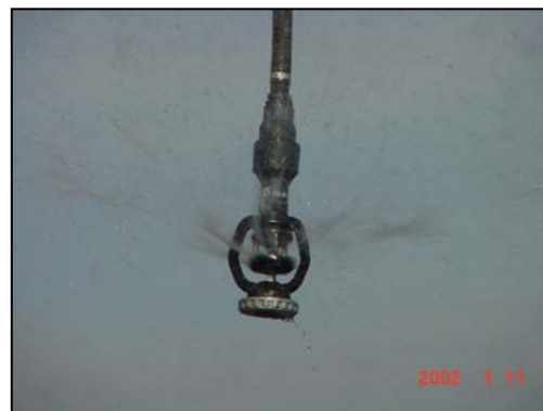
Figure 3 Senninger iWob nozzle during the Mobile Irrigation Lab's efficiency evaluation.
