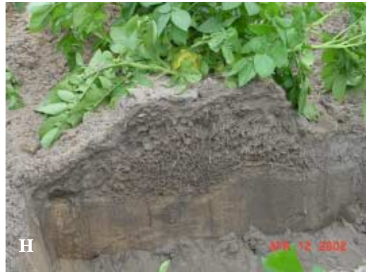
Figure 6 (continued). Use of dye tracer to mimic N and water movement in a potato bed.
