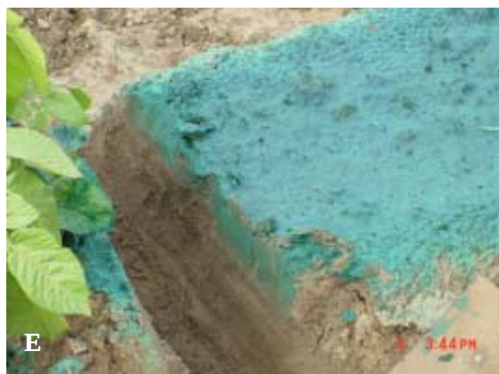
Figure 6. Use of dye tracer to mimic N and water movement in a potato bed.
