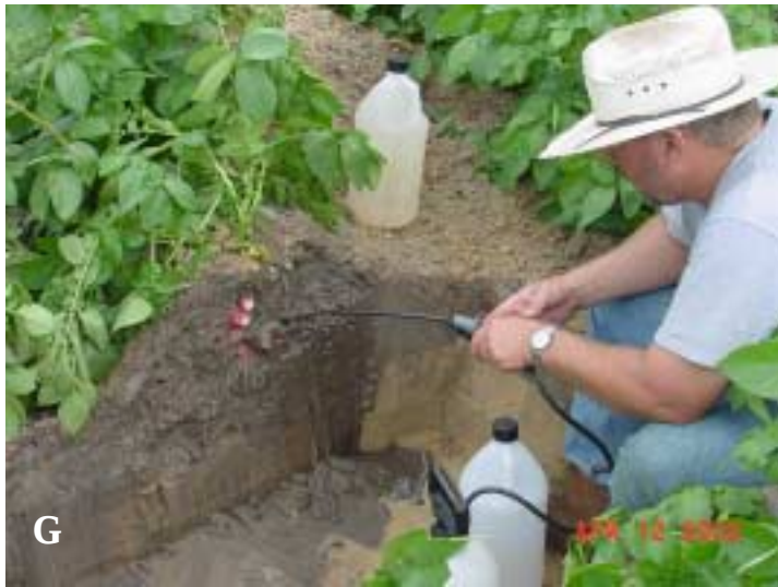
Figure 6 (continued). Use of dye tracer to mimic N and water movement in a potato bed.
