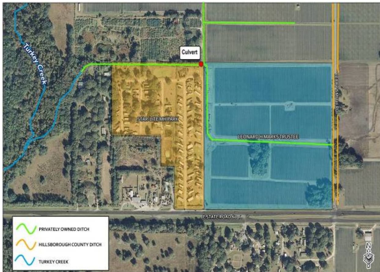
Figure 30. System of conveyances near Jerry Smith Rd and SR 60. The farmers here attribute erosion and sedimentation illustrated in Figures 28 and 29 to the privately owned culvert shown here. Further research is necessary to resolve all concerns and develop an appropriate solution. IFAS and FDACS are in regular contact with the farmers.
