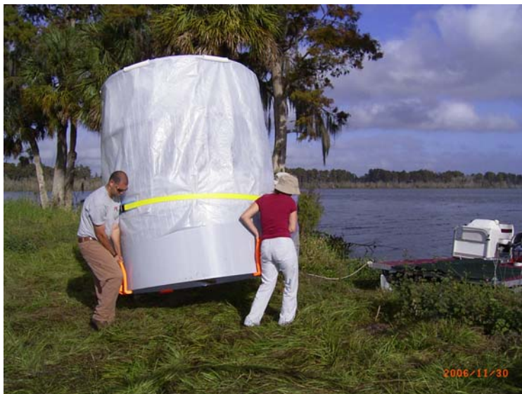
Photo 2. Constructed aluminum mesocosm about to be deployed in Lake Hancock.
