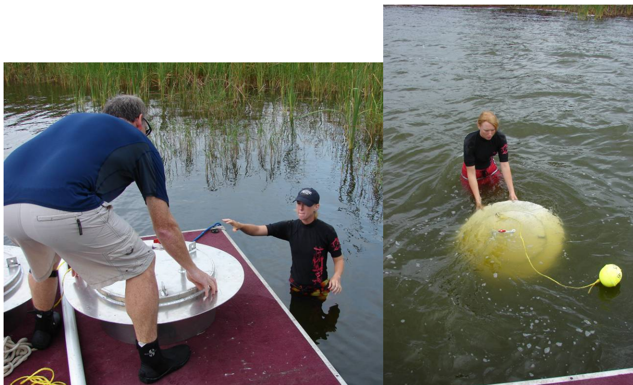
Figure 17. Installation of Groundwater seepage meters
