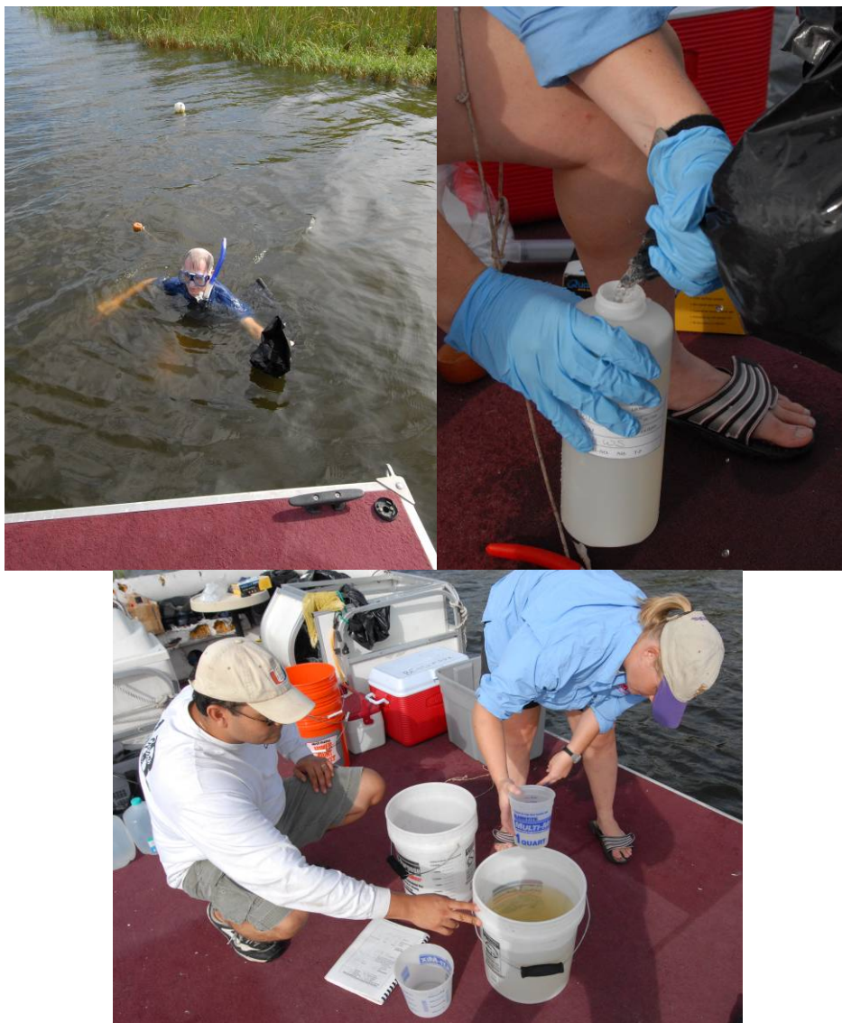
Figure 18. Top Left: Retrieval of groundwater sampling bag. Top Right: Collection of water for water quality analysis. Bottom: Volume determination of groundwater
