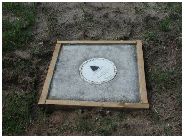
Figure 31. Left- Flush mount groundwater monitoring well. Right- Above-ground groundwater monitoring well
