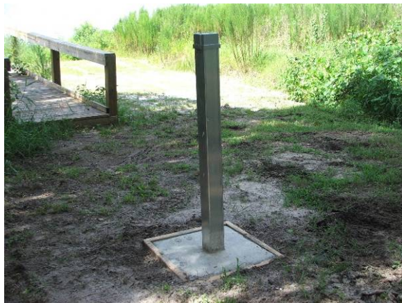
Figure 31. Left- Flush mount groundwater monitoring well. Right- Above-ground groundwater monitoring well
