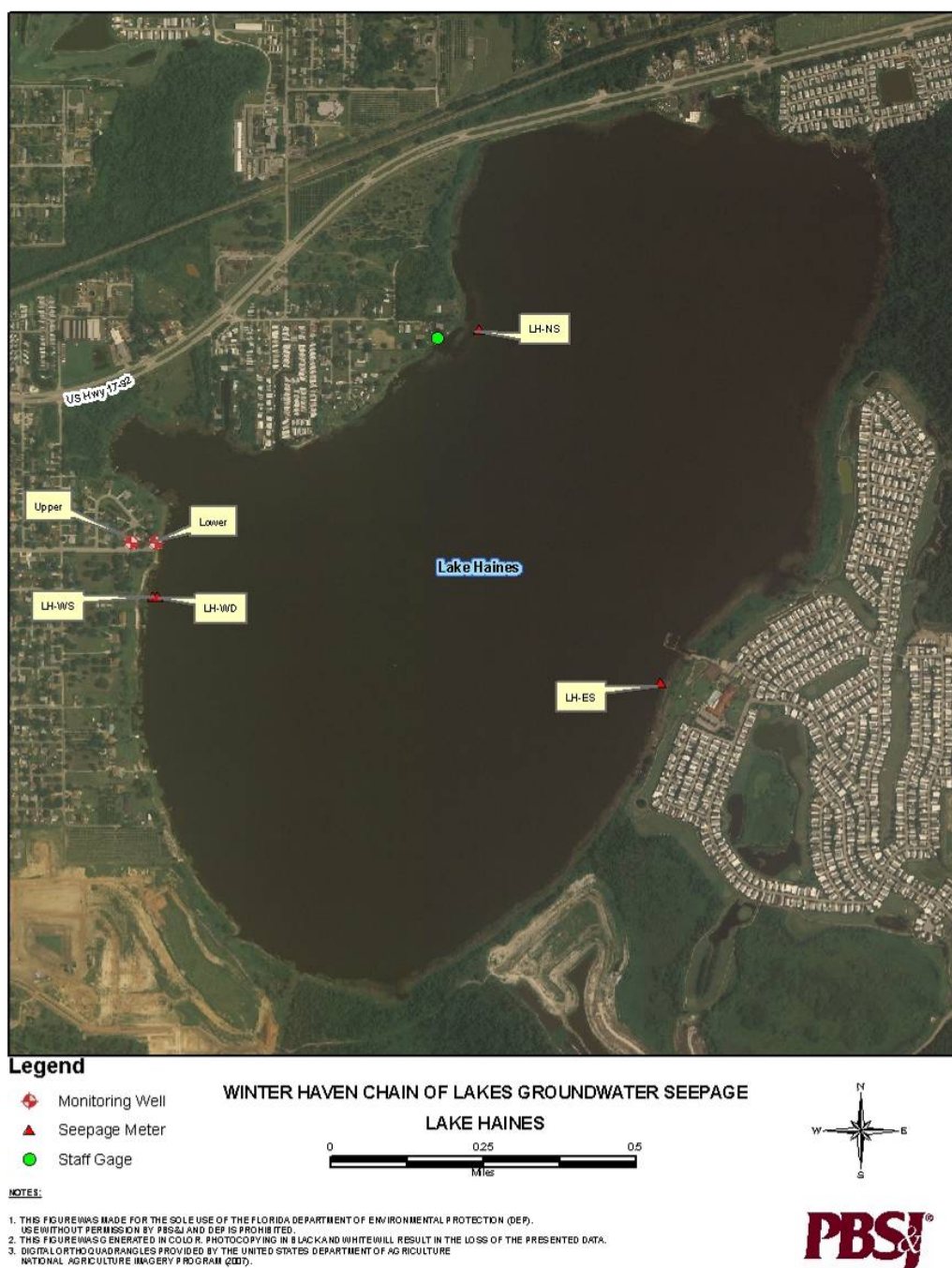
Figure 13. Location of groundwater seepage meters, surficial aquifer monitoring wells and lake staff gauges monitored during the groundwater study in Lake Haines
