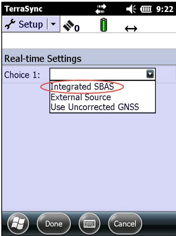
Figure 16. Screenshot illustrating Real-Time Settings subsection of the TerraSync Setup section.
