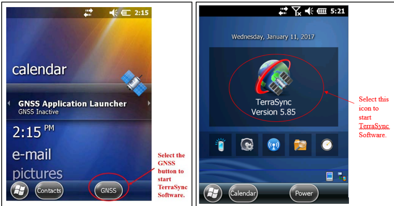
Figure 2. Screenshots illustrating GNSS unit home screen for the GeoExplorer 6000 (left) and Geo 7x (right).
