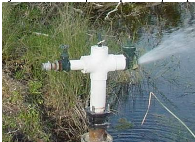
Figure 36. The addition of PVC adapters allows for sampling of certain wells.
