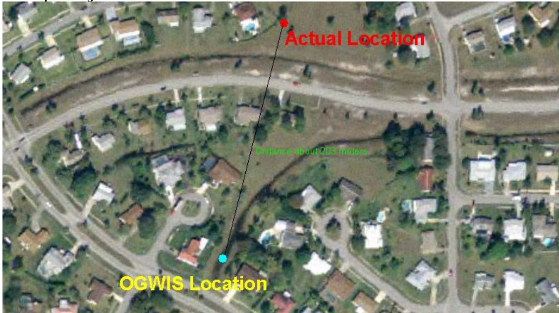
Figure 48. Sometimes a well is not where GWIS shows it to be. However, the nearest adjacent well should never be sampled in lieu of the targeted well.
