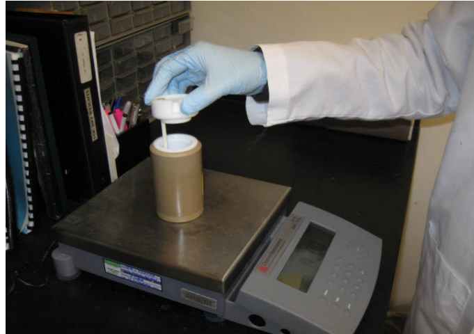
Sample measured into a microwave digestion vessel
