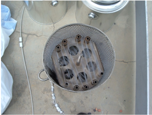
Figure 10. SPMD Membranes in Canister.
