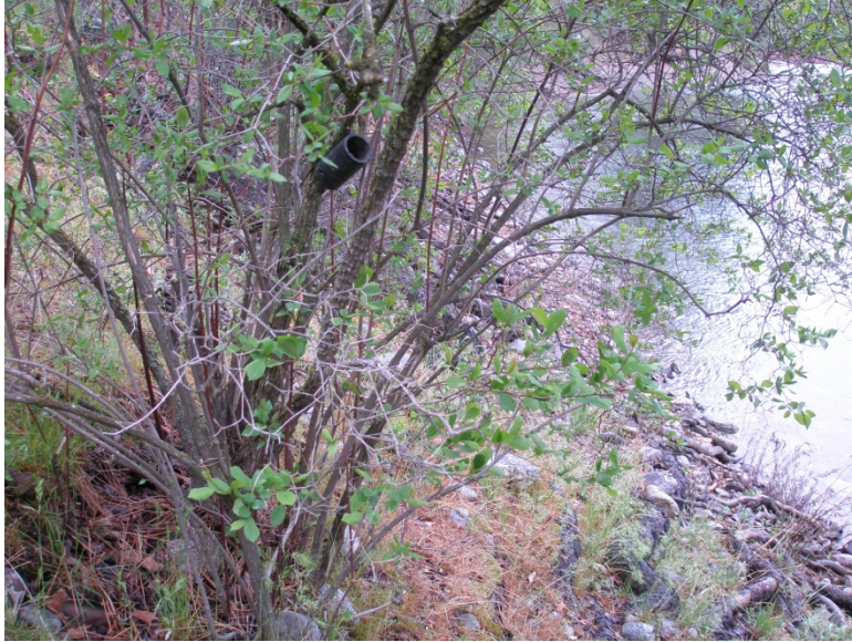
Figure 7. TidbiT™ Shaded in PCV Pipe.
