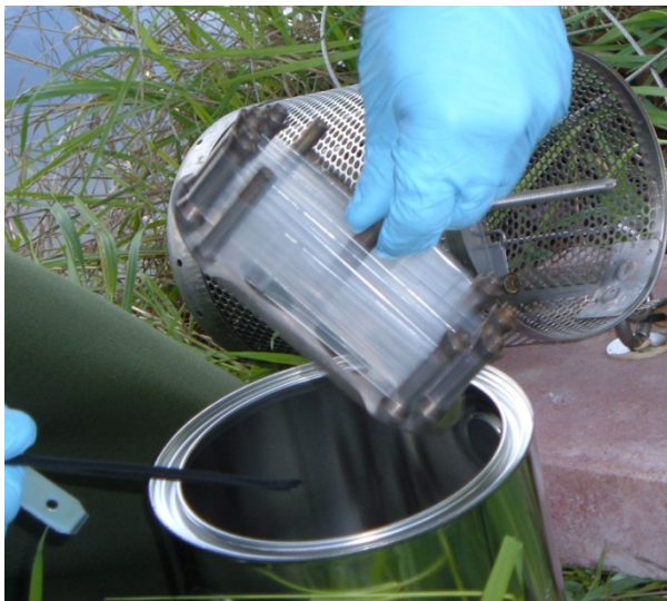
Figure 9. Pulling a Spider Carrier with Membrane Out of the Can.
