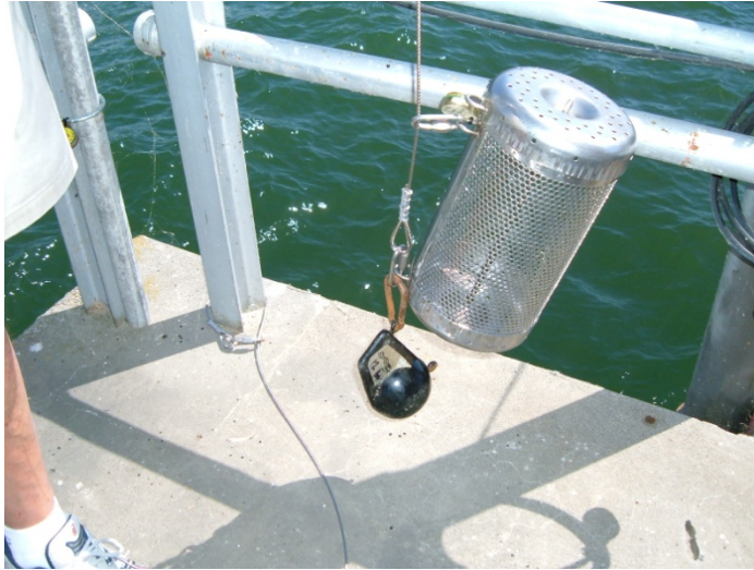
Figure 5. SPMD Sampler Hung off a Dam.
