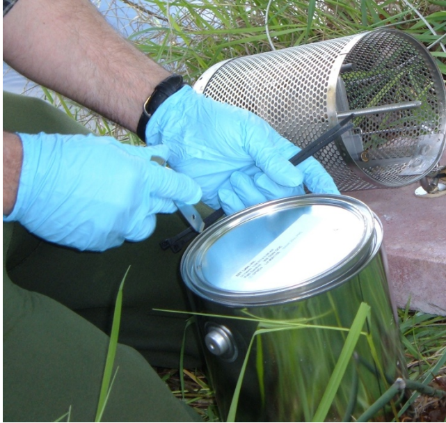
Figure 8. Loosening the Lid of the Can (church key in right hand, zip ties in left hand).
