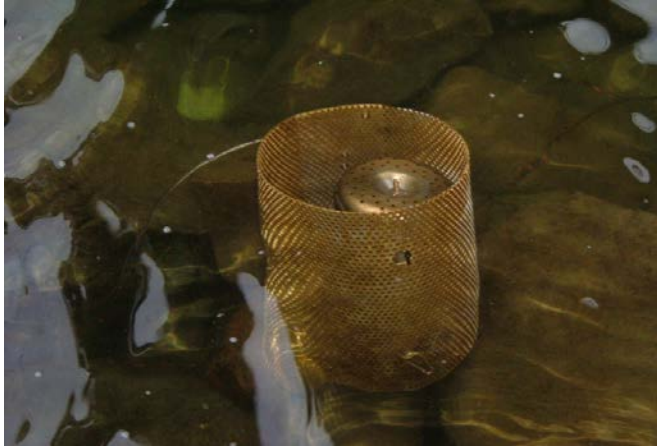
Figure 4. SPMD Sampler in Shade Device Attached to Concrete Block in Water.
