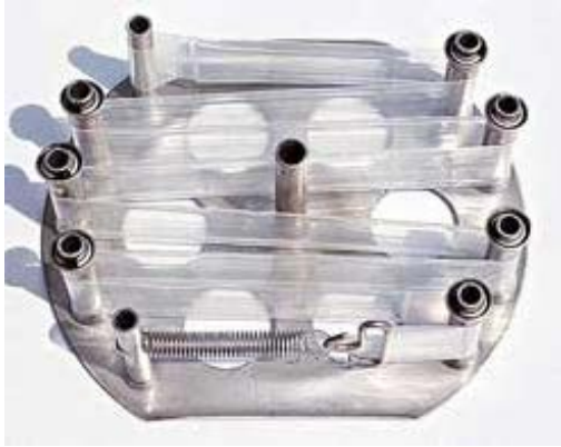
Figure 1. Single SPMD Membrane on a Spider Carrier.
