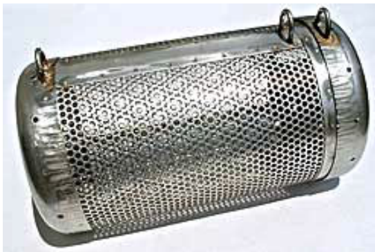
Figure 2. SPMD Deployment Canister (five-membrane capacity).
