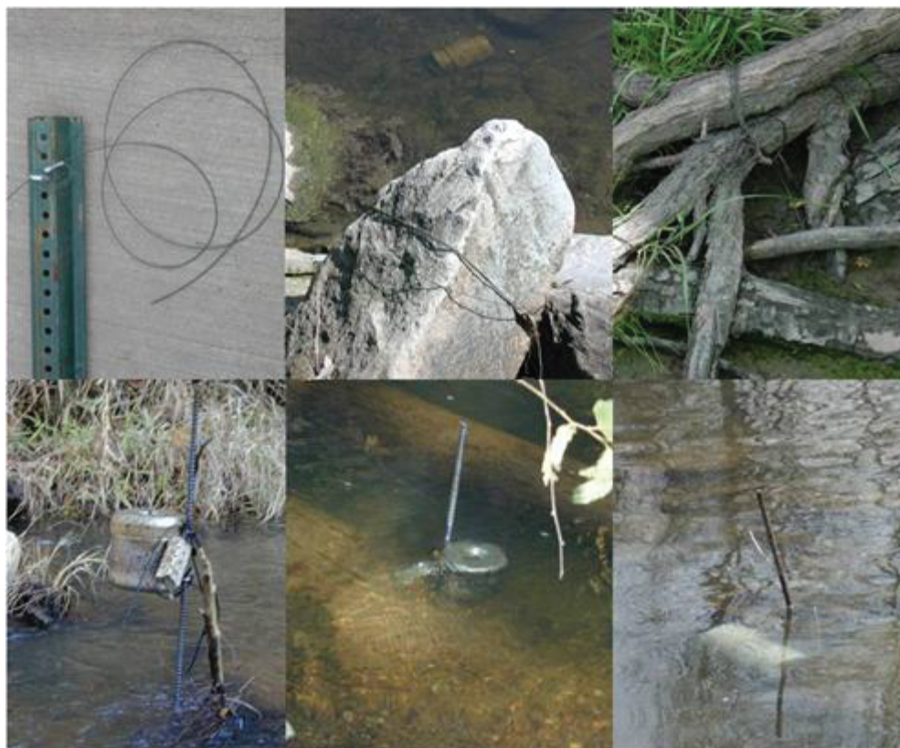
Figure 3. Methods of attaching deployment canisters to shore and mid-channel of streams. Photographs by John Tertuliani, U.S. Geological Survey (top row), Wade Bryant, U.S. Geological Survey (bottom left and center), and Christopher Guy (U.S. Fish and Wildlife Service, bottom right).
