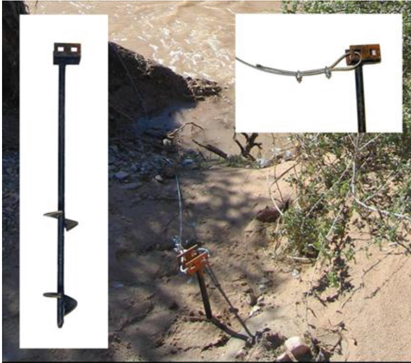
Figure 4. Ground anchors (insets) can be useful for shore deployments when no other structures (trees, fence posts) are available for attachment purposes. Ground anchors are very strong, but may be difficult to impossible to use in rocky soils. Photographs by David Alvarez, U.S. Geological Survey.
