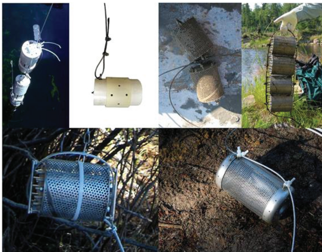
Figure 8. Different options for cabling canisters during deployment in water bodies. Photographs by David Alvarez, U.S. Geological Survey (top far left, top left center, bottom row), Michael Rosen, U.S. Geological Survey (top right center), and Randal Clark, U.S. Geological Survey (top far right).
