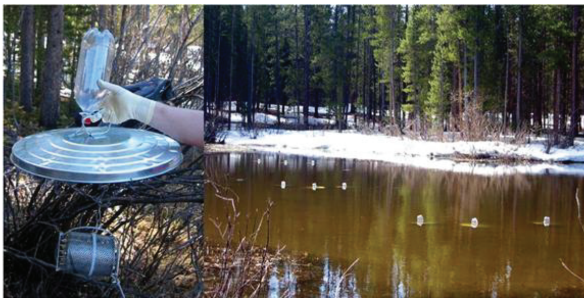
Figure 6. Sunshield used in calm waters to limit potential photodegradation of labile chemicals. Photographs by David Alvarez, U.S. Geological Survey.
