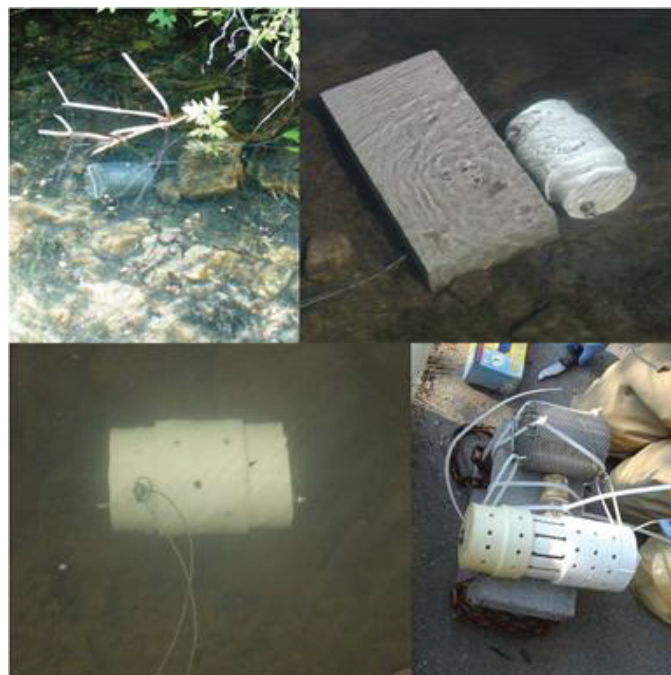
Figure 7. Stream deployments with the deployment canisters cabled to the shore, sitting directly on the streambed, and anchored by concrete blocks. Photographs by David Alvarez, U.S. Geological Survey (top left), John Tertuliani, U.S. Geological Survey (top right, bottom left), and Christopher Guy, U.S. Fish and Wildlife Service, (bottom right).
