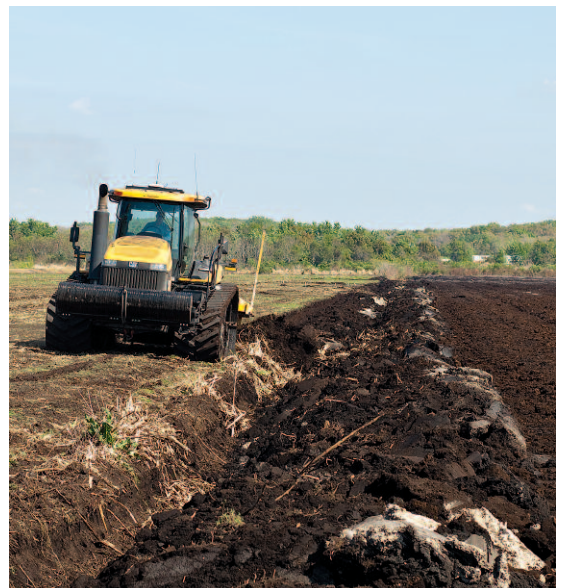
A tractor pulls a special plow that places potentially contaminated soil deep below the surface as part of a soil inversion project.
