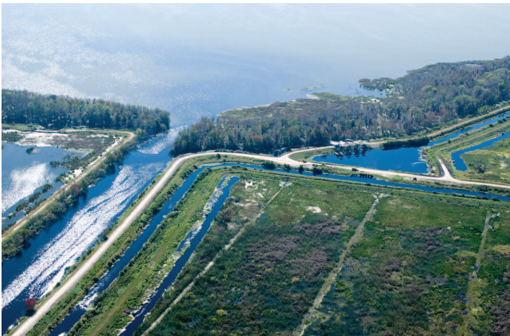
The Lake Apopka Marsh Flow-Way treats water from the lake in wetland cells, releasing cleaner water back to the lake.
