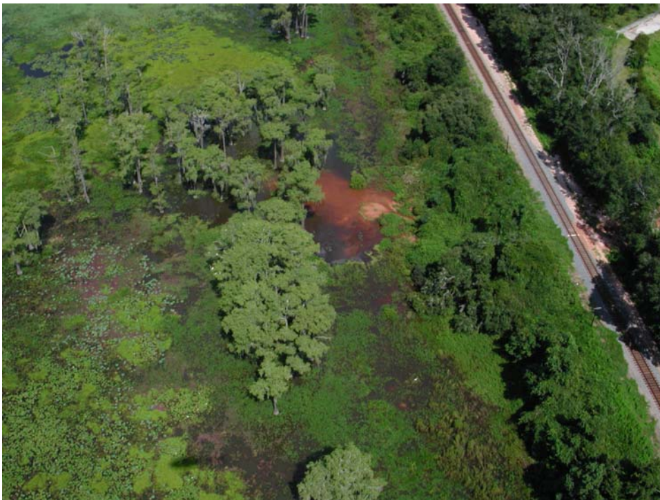
Figure 5.1.2.4: 2002 aerial photograph; Plume in Lake Piney Z from the failed berm.
