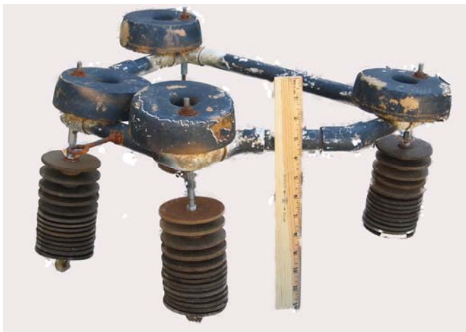
Figure 1. Construction details of the floating Hester-Dendy platform
