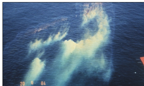
Dispersant field trials in the North Sea. Statfjord crude oil, weathered at sea for 3 hours.
