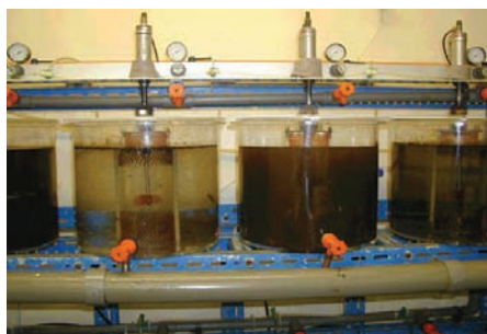
FIGURE 2. A STANDARD SEA TEST IN PROCESS. THE DIFFERENCE CAN CLEARLY BE NOTED BETWEEN MECHANICALLY DISPERSED OIL (LEFT) AND CHEMICALLY DISPERSED OIL (RIGHT).
