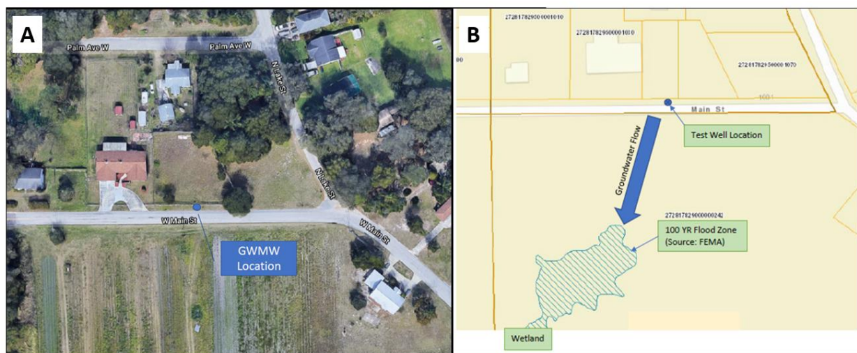
Figure 2. Study site in Lake Hamilton, FL, showing A) aerial imagery of the residence where the Distributed Wastewater Treatment Unit (DWTU) and groundwater monitoring well were installed in Lake Hamilton, FL and B) groundwater flow at the study site.
