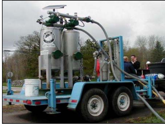
Sand Media Particulate Filter (Source: http://www.spillcontainment.com )
