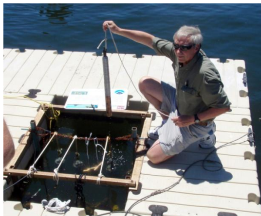
Long-term side-by-side studies comparing water quality data collected by EXO and 6-Series sondes in variable field conditions.
