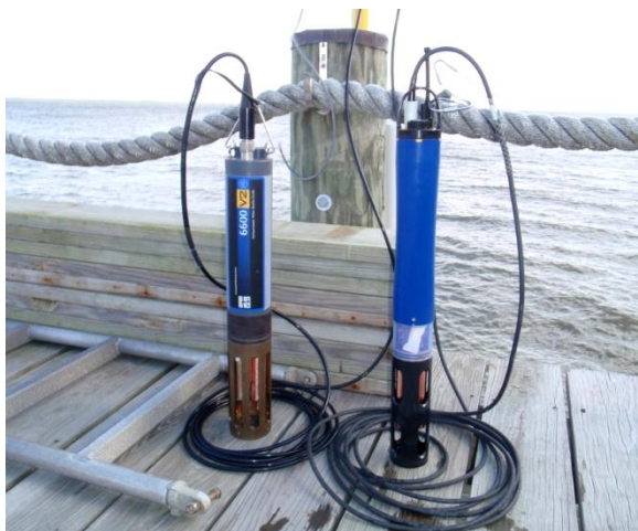
Long-term side-by-side studies comparing water quality data collected by EXO and 6-Series sondes in variable field conditions.
