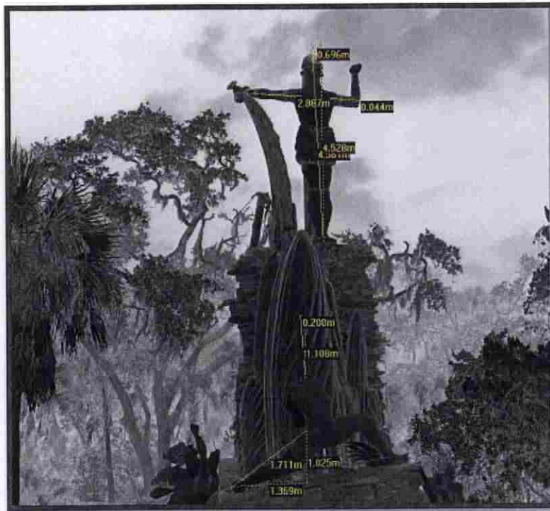
Figure 153. Point cloud derived from the 3D Terrestrial Laser Scan Survey of Tomoki Statue showing as-built detail and measurements
