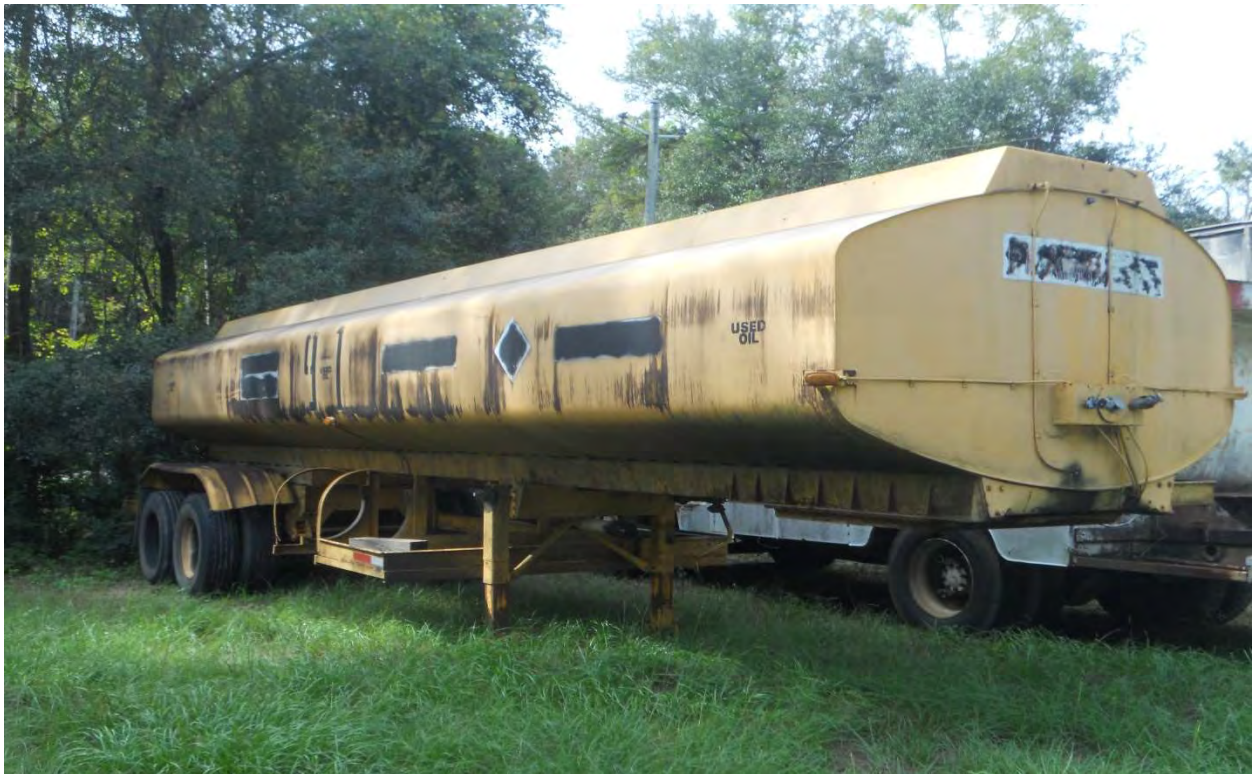
6,400 gallon tanker used for delivery of processed oil and as emergency storage
