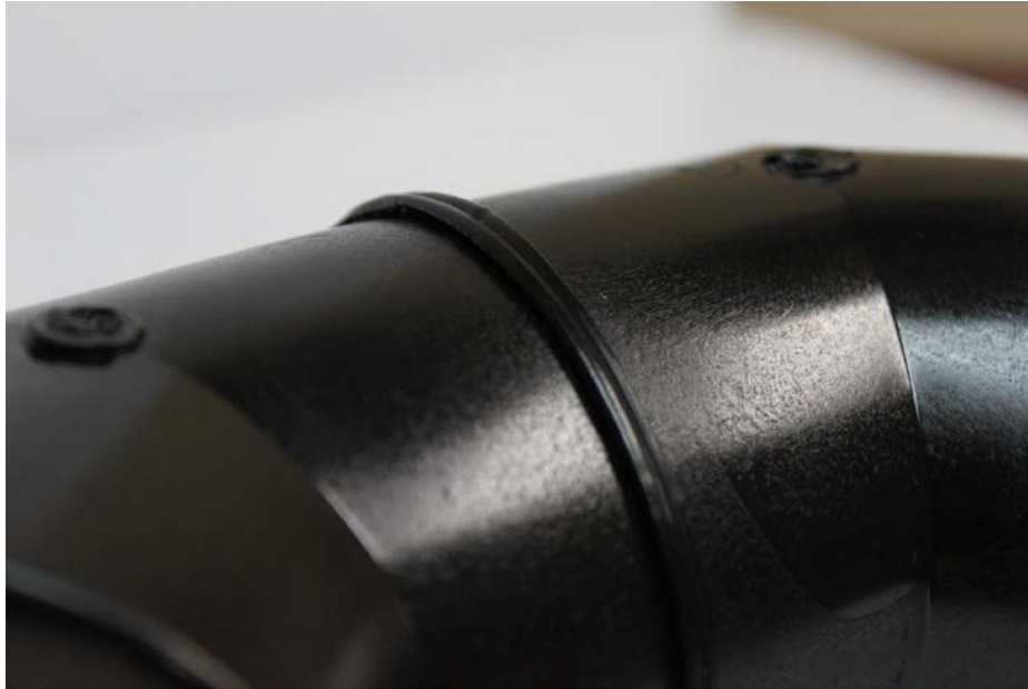
Close up of molded fitting to fitting weld, bead height approx \frac{1}{16} "- \frac{3}{32} ", with approx \frac{1}{32} " deep notch between beads. Both beads have nice rounded edge.
