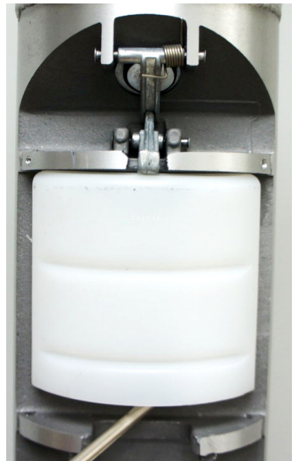
Secondary Float (manually raised) closing the drain lever and stopping flow through the drain valve
