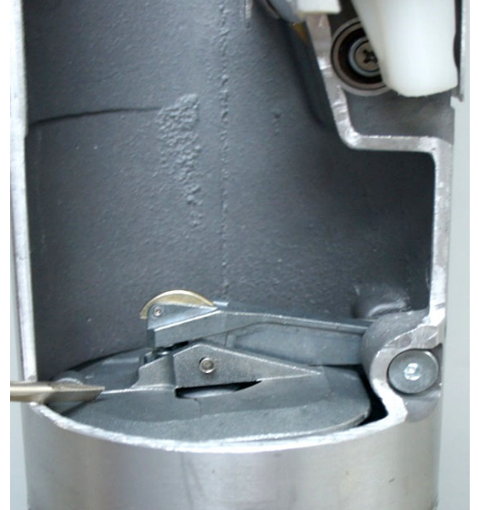
Flapper valve shown closed against viton seal
