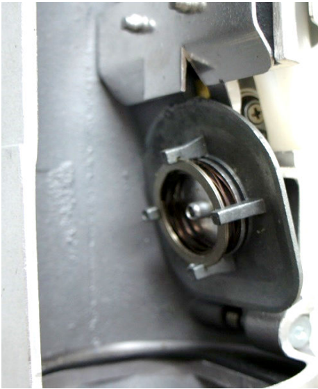
Flapper valve (normal position)
