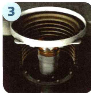
Replace Bellows, Reinstall Upper and Lower Rings
