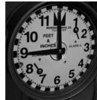
FIGURE 5: Hold thumb nut at desired trip point. Example- Alarm set point at 9 feet - 0 inches.
